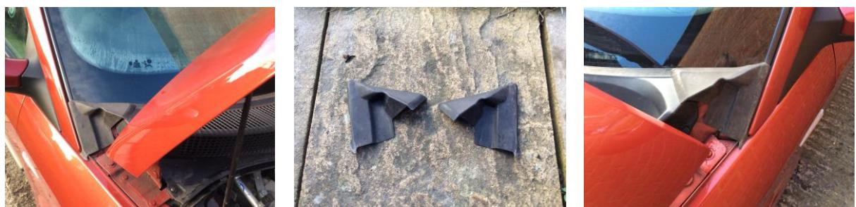
For good measure, remove and clean the strange rubbery ducting dirt trap type things just below the bonnet hinges:
