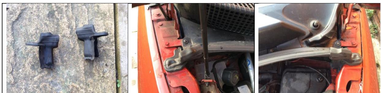
Then remove the rubber seal along the edge by the wipers.
