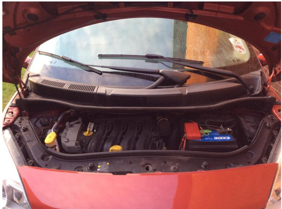
Now, either end of the rubber seal are two "end sealers". Remove them both. They should just pull out. Then remove the long rubber seal along the edge, it should just pull off.
