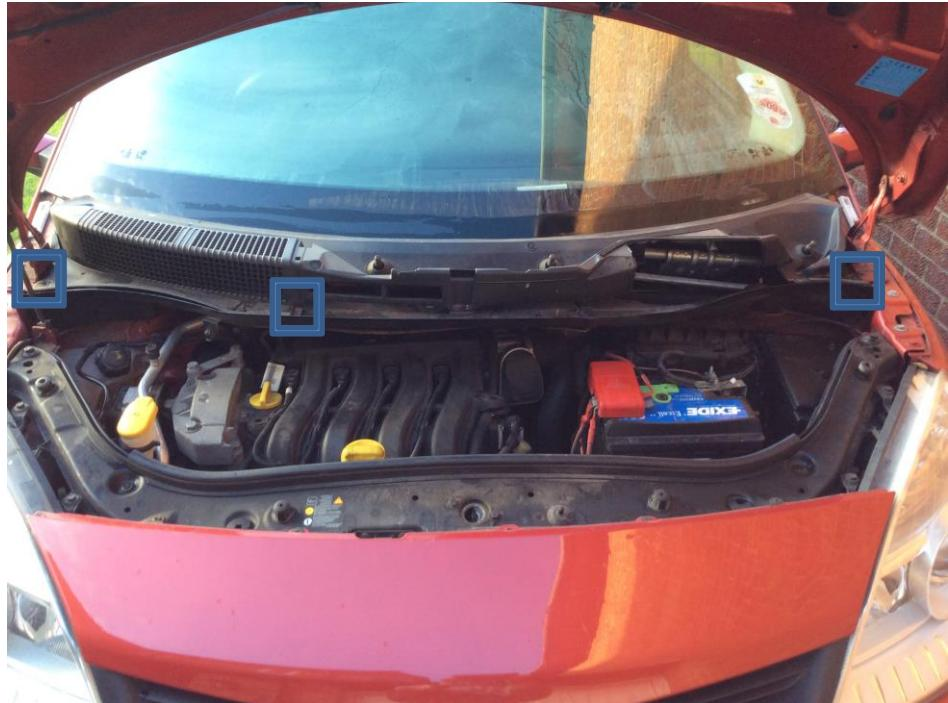
Now, we can clear thing out. On the left, under the windscreens, behind whst I guess is the top of the suspension, you will see a rubber top of tube. Clean around it and try to make sure that the top of the tube (ie. The entry) is completely clear. In the end I resorted to shoving a finger down the tube to unblock it. Seemed to work.
