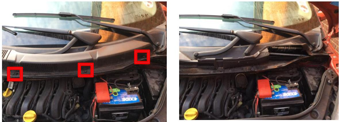
To stop them getting in the way later, remove the bits of plastic at either end of the main plastic holder:
