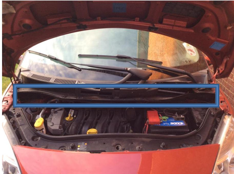
Looking closely just below the wipers, you will see a piece of plastic. Undo the three nuts (10mm hex) holding it in place and remove it:
